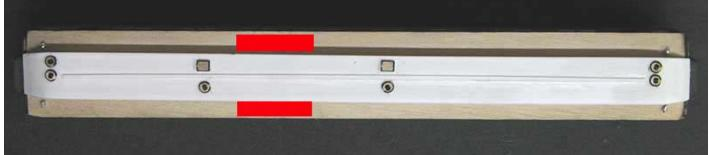
Completed roof before painting. Red indicates battery box location in the underframe in relation to roof orientation.
