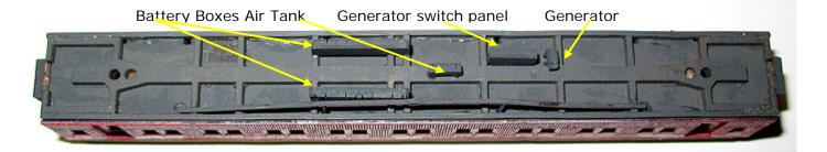
Above is a view of underframe details. Note one truss rod was removed for photographic purposes.
